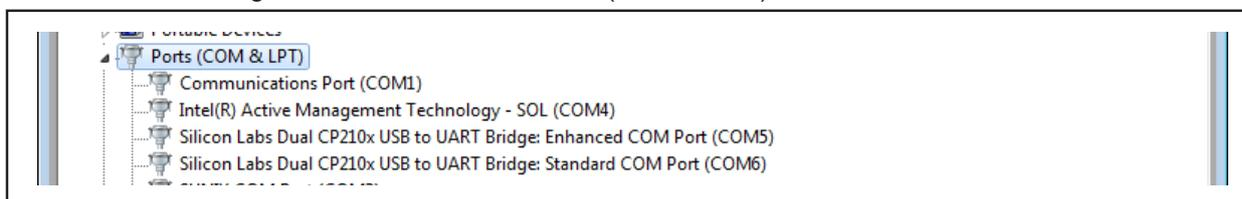
"Silicon Labs Dual CP210x USB to UART Bridge : Enhanced COM Port (COM\*\*)"
